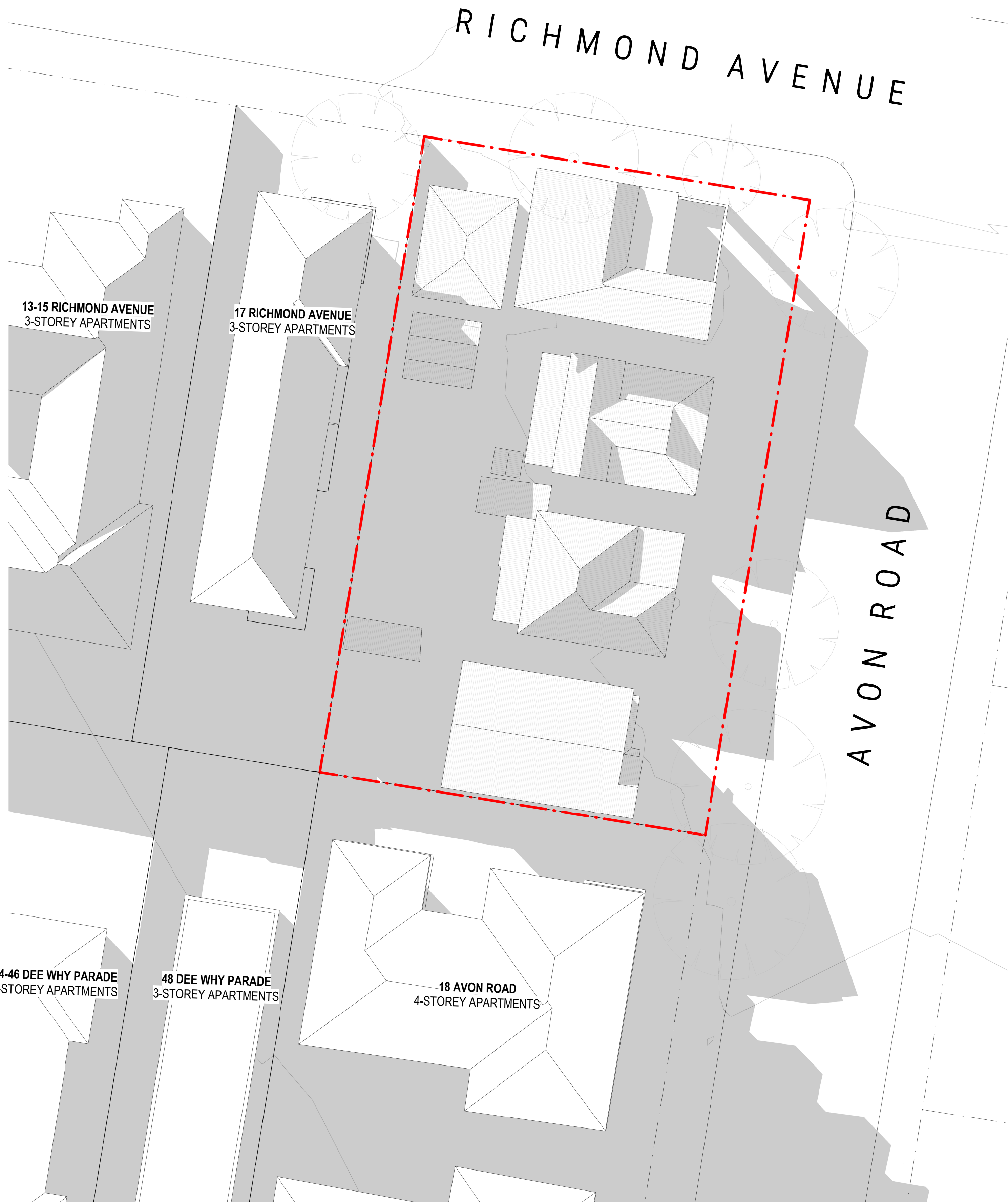
1 EXISTING SHADOW DIAGRAM - 3PM JUNE 21ST DA503 1:200 @ A1
