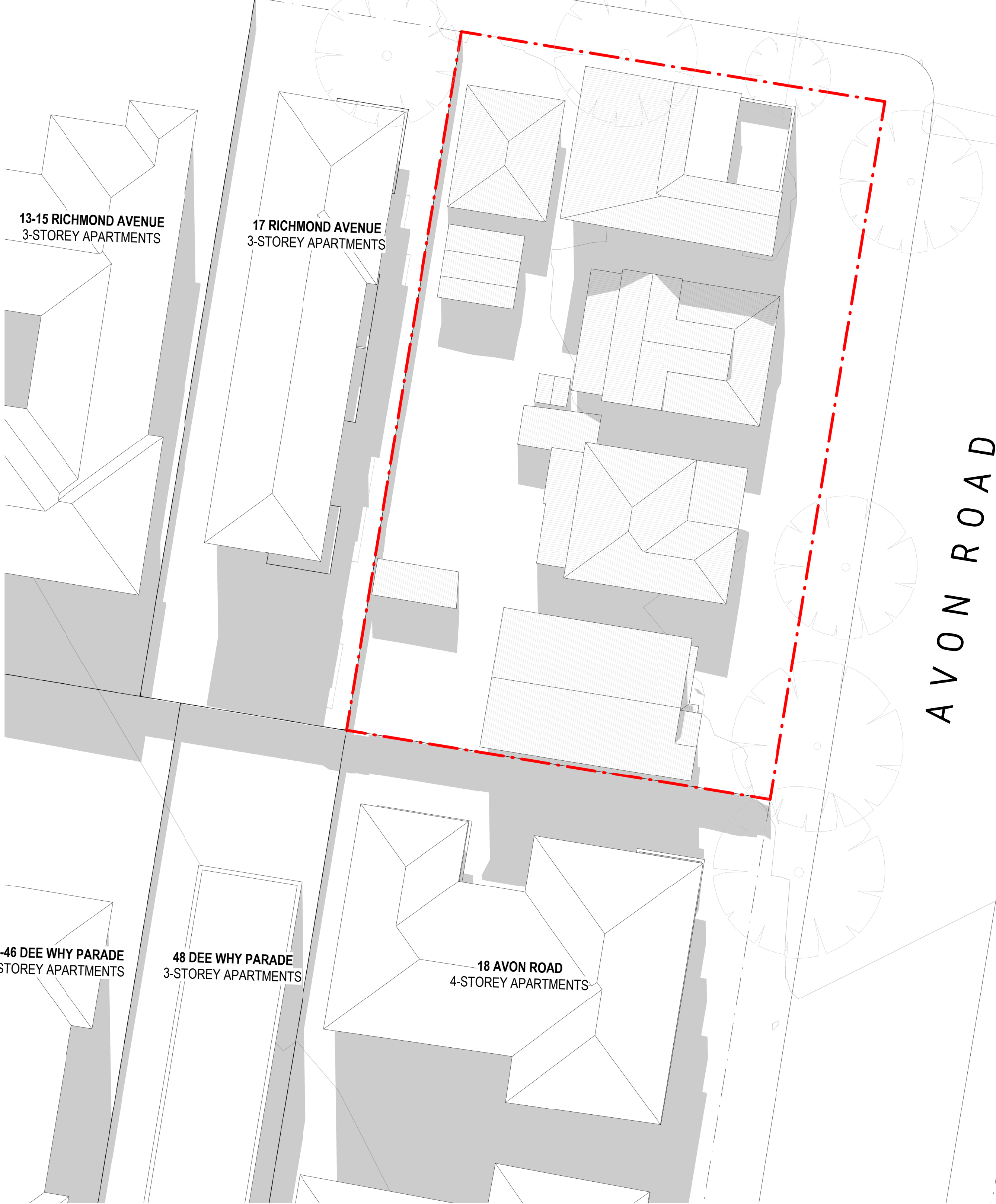
1 EXISTING SHADOW DIAGRAM - 12PM JUNE 21ST DA502 1:200 @ A1
